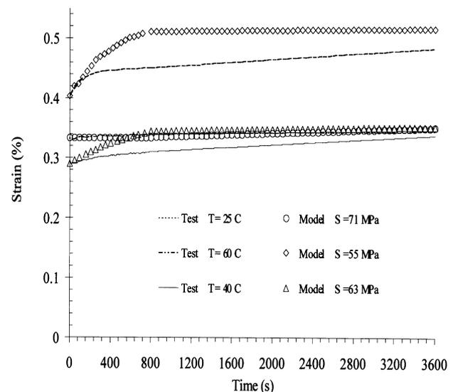
Fig. 4. Comparison of test results and model predictions for creep tests at three temperatures.
