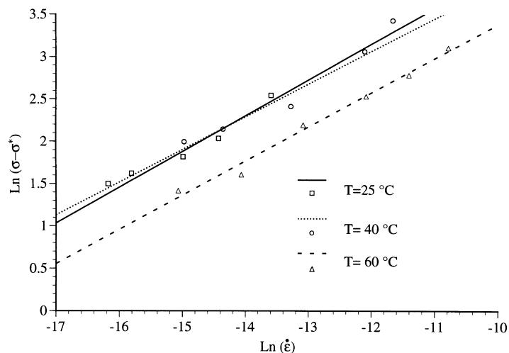
Fig. 2. Logarithm of overstress versus logarithm of strain rate at three temperatures. These curves are used to determine the material constants,  $K$  and  $m$ , at each temperature. Overstress is in MPa.
