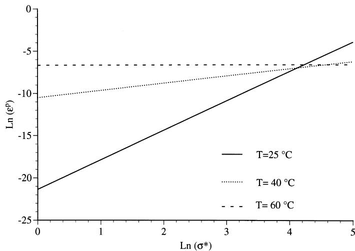
Fig. 3. Logarithm of plastic strain versus logarithm of quasistatic stress at three temperatures. These curves are used to determine the material constants,  $A$  and  $n$ , at each temperature. Quasistatic stress is in MPa.
