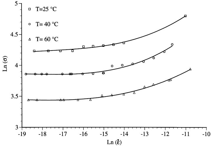
Fig. 1. Logarithm of the stress versus logarithm of the strain rate at three temperatures. Stress is in MPa.
